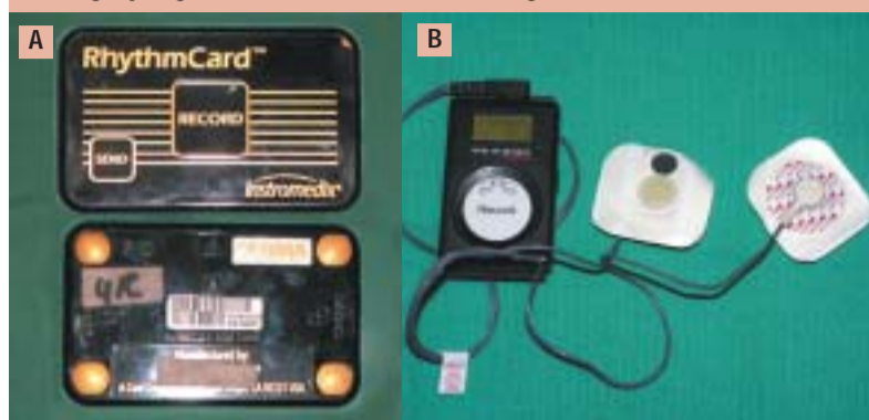
Figure 8: External event monitors. A. The 'RhythmCard' (top and bottom). It is slightly larger than a credit card. B. The 'King of Hearts' event monitor.
